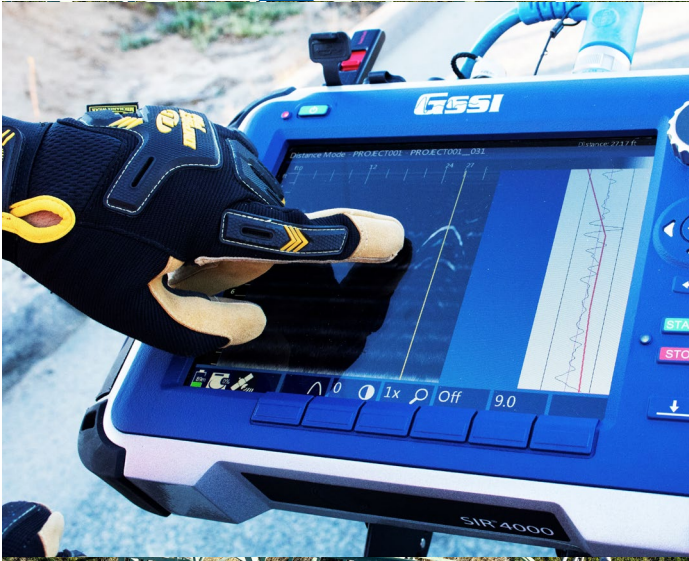
Locating an existing water main with GSSI Ground Penetrating Radar (GPR).
