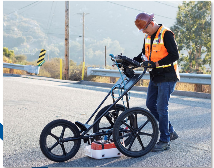
GPR utility locating – identifying water, gas, electric, TELCO/CATV, and sewer/storm drain locations.
